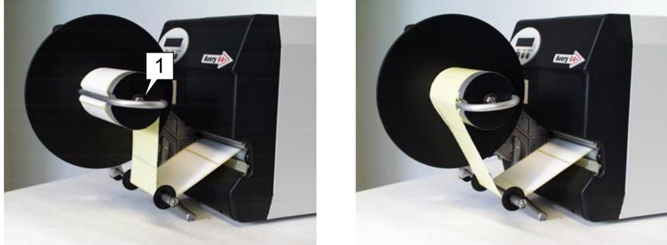
Fig. 5 Left side: direction of rotation = left (labels outside); right side: direction of rotation = right (labels inside)
