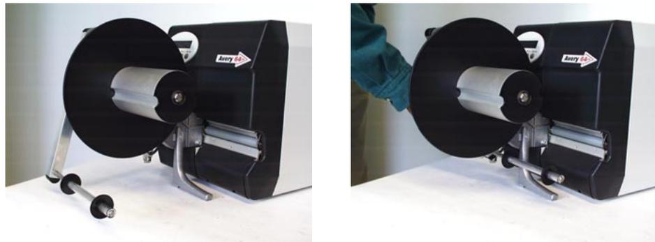
Fig. 4 Left side: bouncer arm in zero position; right side: bouncer arm in final position.
